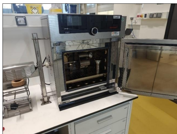
Figure S1.1. The setup used during the hydrothermal synthesis of W/ VO_2 particles. Left: a wide-angle view of the furnace, highlighting its design, including a rotating device. Right: a detailed photo showing the arrangement of autoclaves within the furnace, showcasing both vertical static and horizontal rotating configurations.
