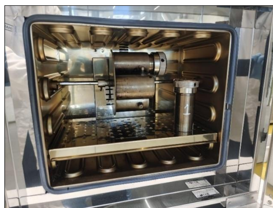
Figure S1.1. The setup used during the hydrothermal synthesis of W/ VO_2 particles. Left: a wide-angle view of the furnace, highlighting its design, including a rotating device. Right: a detailed photo showing the arrangement of autoclaves within the furnace, showcasing both vertical static and horizontal rotating configurations.
