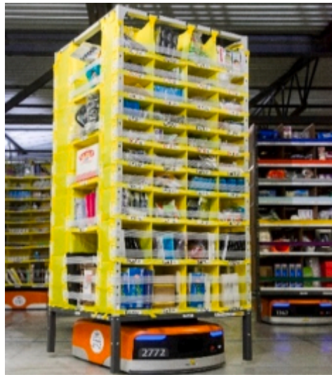
Figuur 11: Automated guided vehicle / autonomous mobile robot (Mirzaei et al., 2021)
