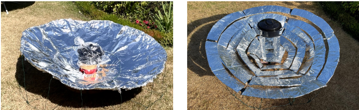
Figure 5: Visual representation of the locally made parabolic prototypes included in the study, referred to as prototype 2/3 (left) and prototype 4 (right).
