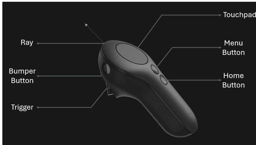
Figure 3.5: Mapping of the AR controller inputs of the Magic Leap
