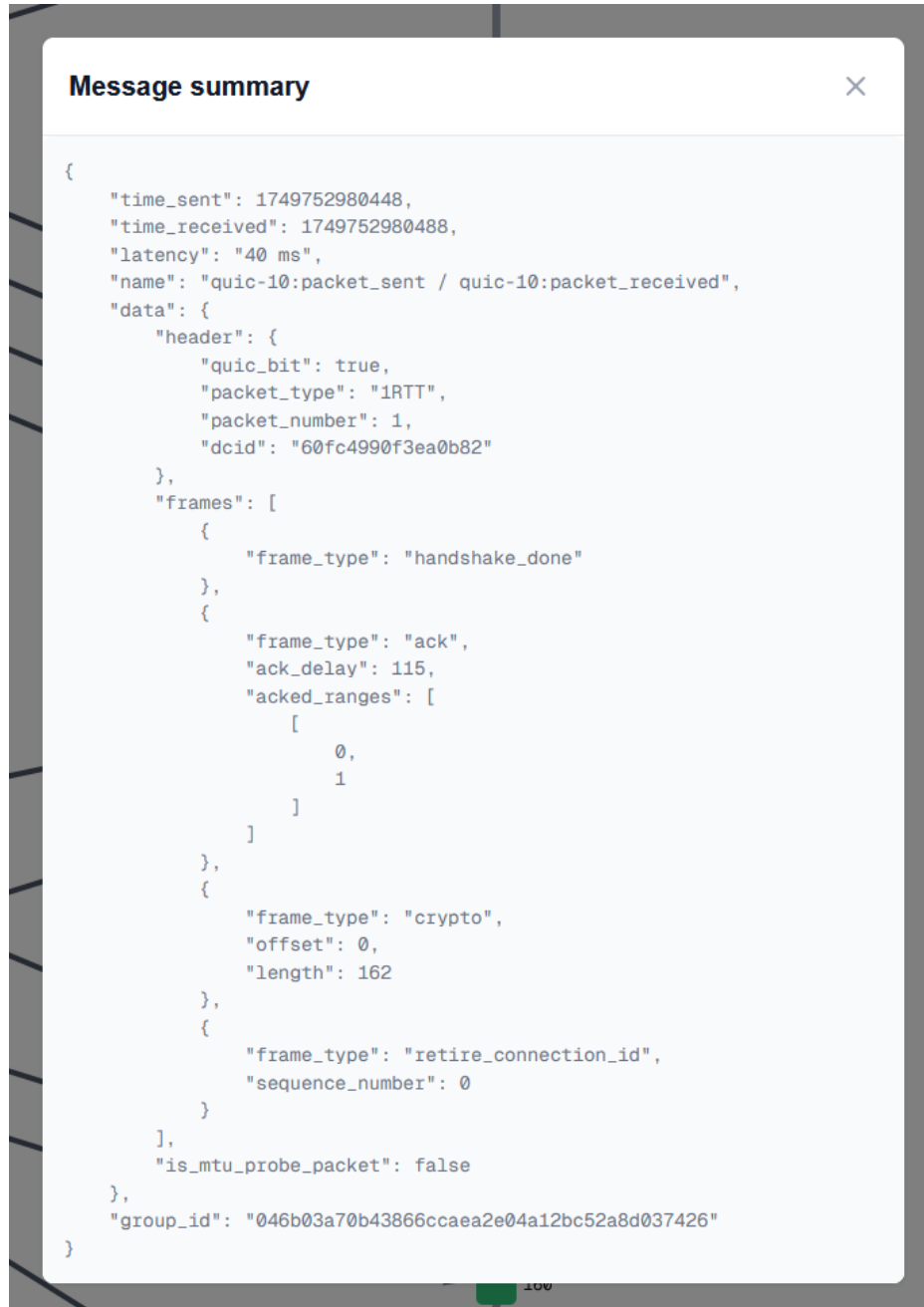
Figure 4.10: Example of a message summary showing the sent time, received time, latency, names of both events, and the common data
