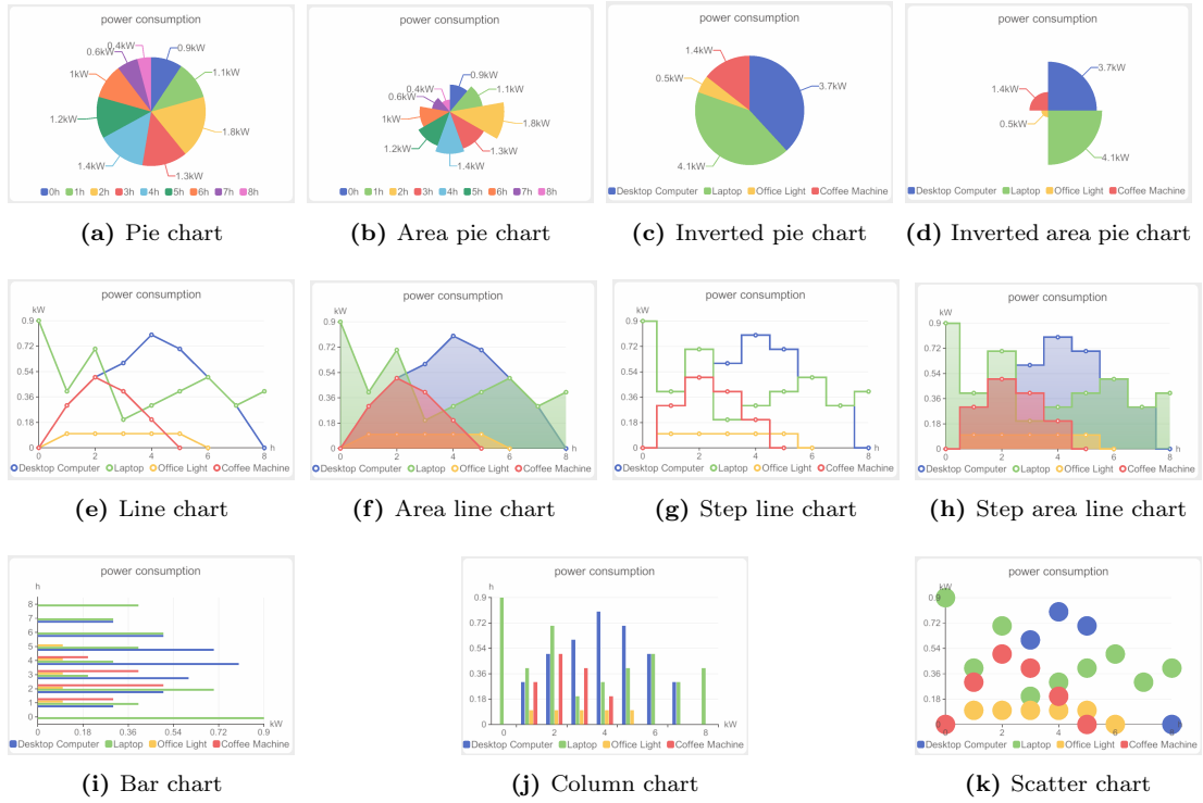
Figure 4.18: All the available recommended visualisations for composite continuous data (multiple components & single data option). In this case, the composite continuous visualisations are for four different components: desktop computer, laptop, office light and coffee machine. They visualise the power consumption, which is continuous data.
