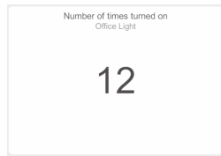
Figure 4.16: The only available recommended visualisation for single discrete data. It shows the number of times the office light has been turned on.
