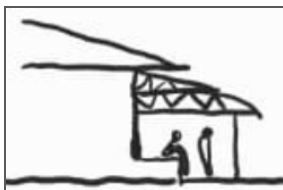
c. A canvas roof added onto a metal roof.
