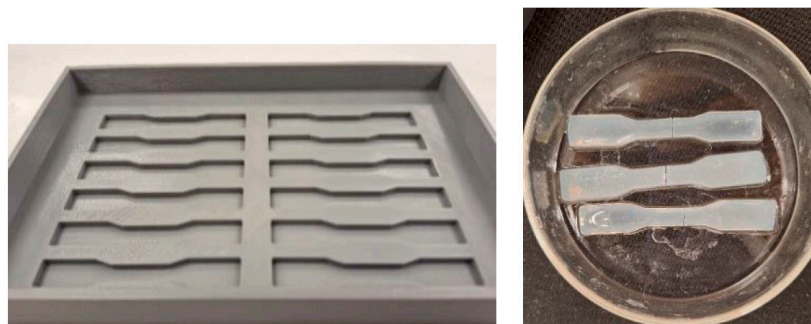
Figure 13. Dog-bone-shaped mold and sample for tensile test.
