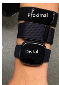
Figure 2. Placement of the wrist-worn wearable devices. A rotation scheme was applied. The wearables were worn as close as possible to each other. The most distal wearable was worn just above the wrist bone.
