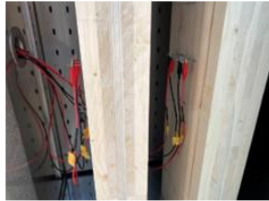
Fig. 3: Continuous measurement of steel-timber connection in climate chamber
