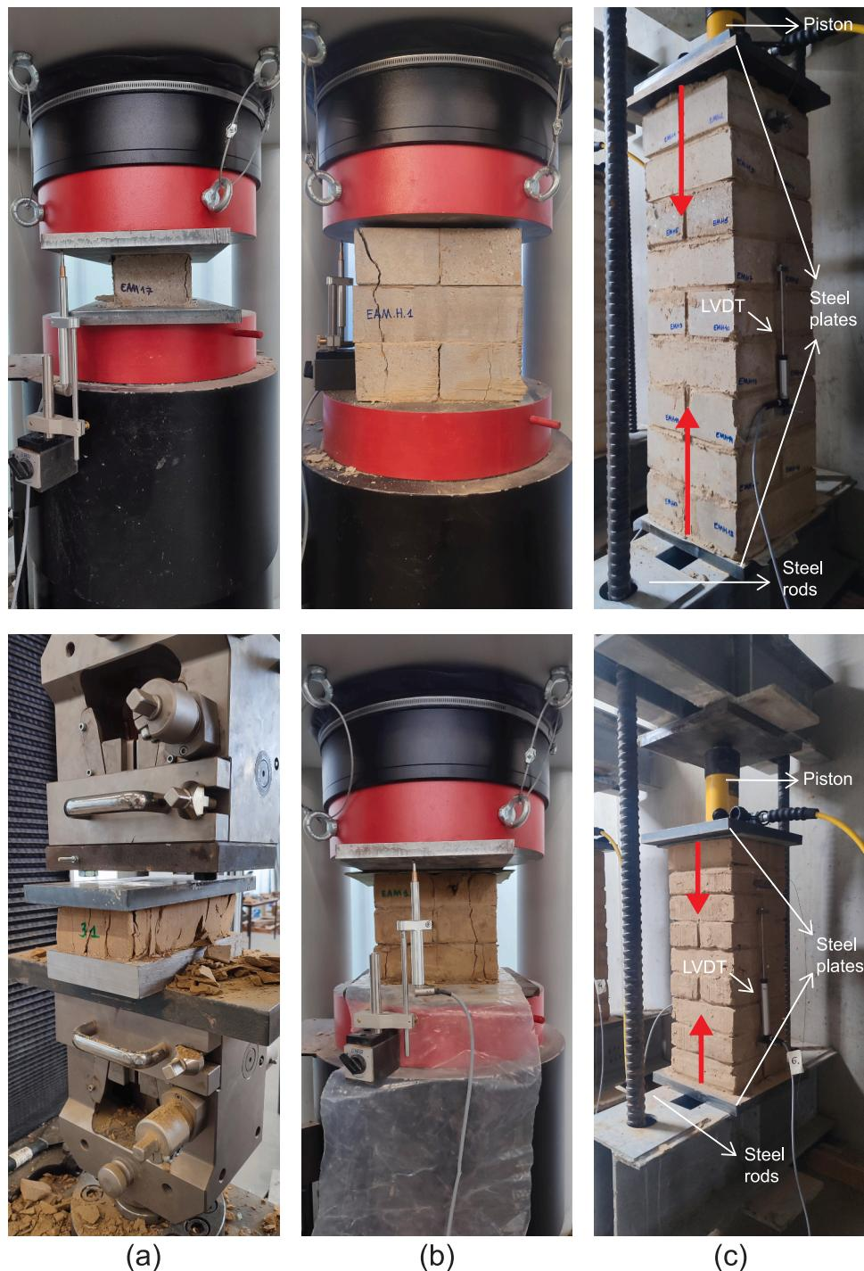
**Fig. 3.** Experimental setups with CEBs (top) and MEBs (bottom) to determine (a) the compressive strength of new and reclaimed earth blocks, (b) the compressive strength of earth block masonry columns, and (c) the sustained loading of the earth block masonry columns.
