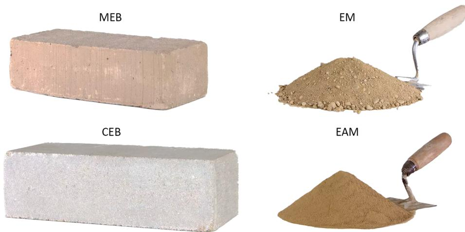
**Fig. 2.** A non-stabilised moulded earth block (MEB) and a cement-stabilised compressed earth block (CEB) were combined with an earth mortar (EM) and a thin-layer earth adhesive mortar (EAM) (© photos by BC Materials).
