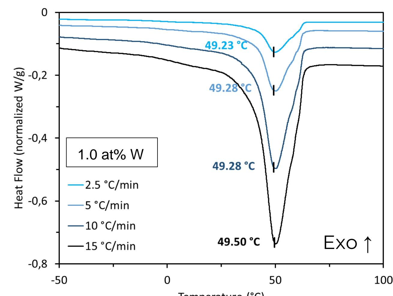
DSC was performed at multiple heating rates (2.5–15 °C min<sup>-1</sup>) for W-doped VO<sub>2</sub>.
