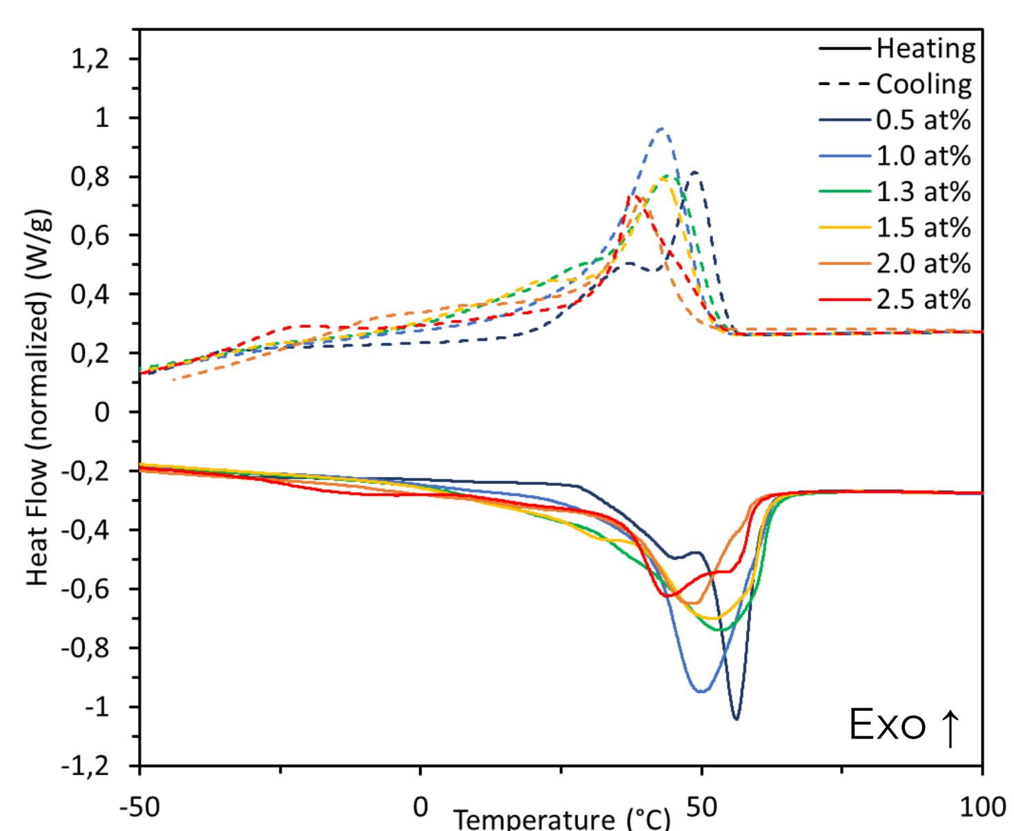
**Increasing W content lowers the VO<sub>2</sub> switching temperature**, though the reduction is smaller than expected due to:
