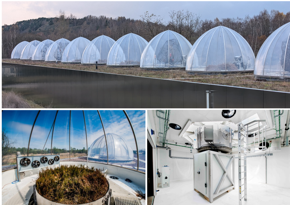
Figure 1.2: Upper picture: an outside view showing a subset of the Ecotron units with the National Park in the background, some units contain heathland, others contain pear trees. Bottom left picture: view inside the dome; on the center left one can see the black fans replicating wind flow on the basis of real-time measured data, a heathland extract of the National Park has been put in a lysimeter (the cylindrical iron tube). Bottom right picture: ground level view of an Ecotron unit; the lysimeter is shown in more detail including cabling for the measuring devices, the black fans in the ceiling control the temperature in the dome. Bottom pictures are courtesy of the UHasselt Field Research Center.
