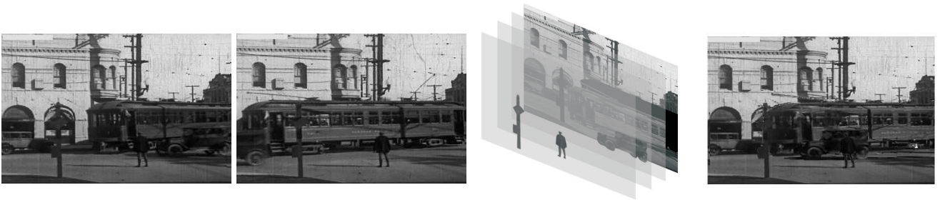
Figure 1: From left to right: (a) and (b) The leading and trailing frames. (c) The layered representation. (d) The reconstruction of an intermediate frame. Notice the occlusions by the road sign and the human figure.
