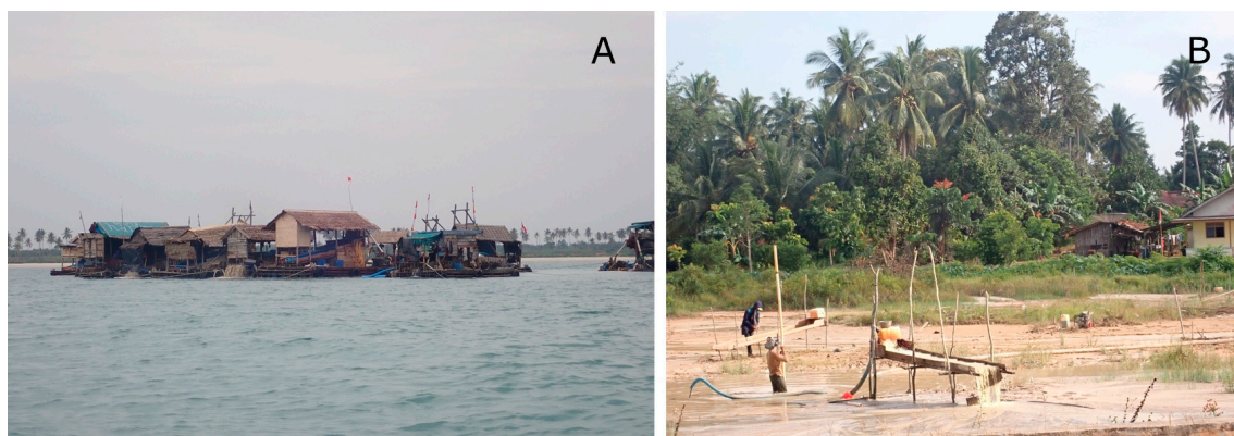
Figure A5. ‘Unconventional tin mining’ operations on Bangka Island: (A) Offshore platforms extracting tin sand from the seabed (Jebu Laut, 25 August 2021); (B) Onshore tin washing process, where tin sand is washed to separate tin from other materials (Bangka Tengah Regency, 9 August 2022); Photos by Suci Puspita Sari.
