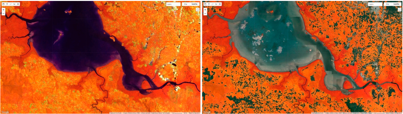
Figure A3. Comparison of false color composite images: initial (left) and after applying elevation masking and filtering criteria (right) to focus on mangrove regions.
