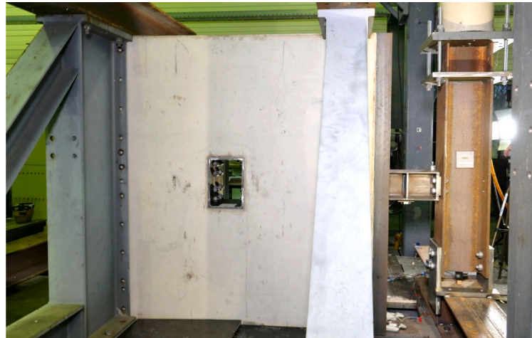
(g) Assembly of the test setup, including the HCW_C-2 specimen
