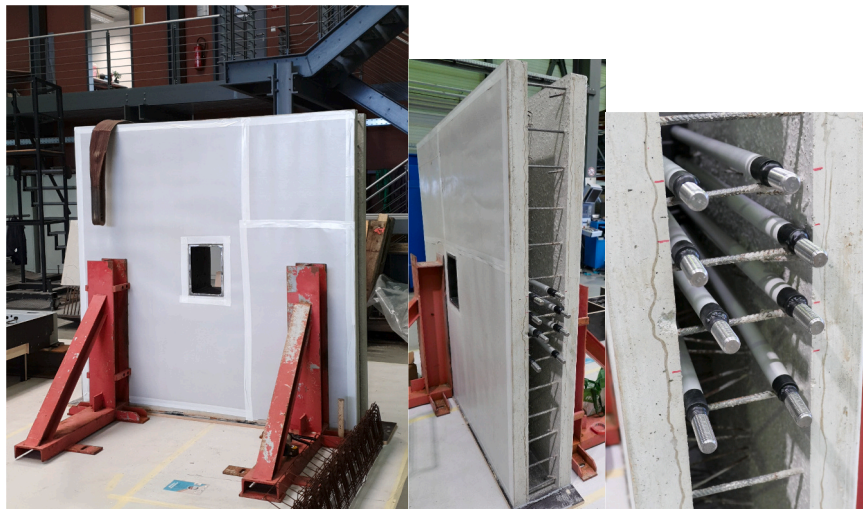
(b) Positioning of the RHS at wall center and of the threaded rods
