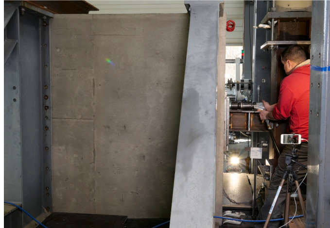
(g) Assembly of test setup and post-tensioning of the threaded rods using a pneumatic torque wrench
