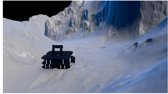
Figure 3: Simulated robot on a lunar-like terrain. Terrains were generated from displacement maps and used for both rendering and physics simulation.
