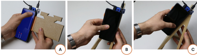
Figure 8: Using the StoryStick++ core unit to measure (a) the length of an object, (b-c) the angle between two sides of an object.
