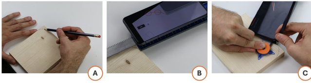
Figure 5: Rounding the edges of the roof panels of the birdhouse by (a) making a freehand sketch of the rounded corner, (b) capturing the sketched arc by sampling 3 points with StoryStick++, (c) plotting the redefined arc on all corners of the roof.
