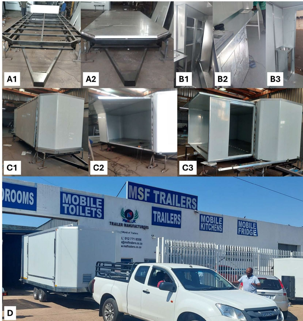
254 255 Figure 3: Construction of the trailer that would be converted into a mobile laboratory, showing 256 the trailer's (A) chassis and floor, (B) stainless steel interior cabinets, (C) ET room extension 257 with roof and side panels in the open and closed positions, and (D) the fully constructed trailer. 258
