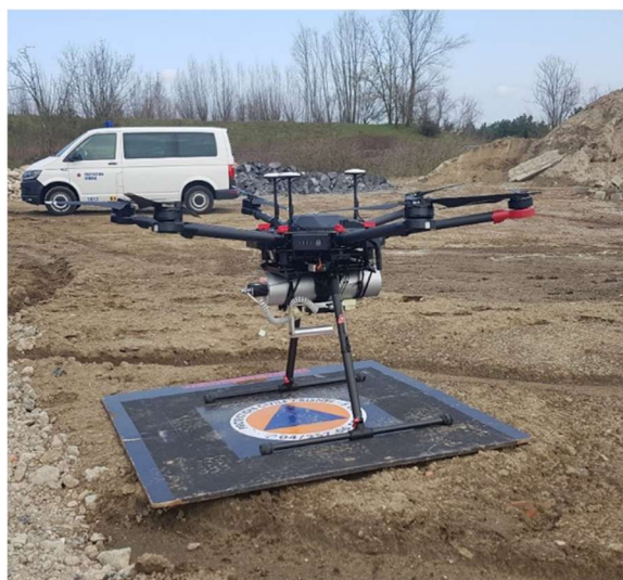
Figure 25: DJI M600 Pro with the Automess 6150AD-b payload (including smartphone and Bluetooth module) underneath.
