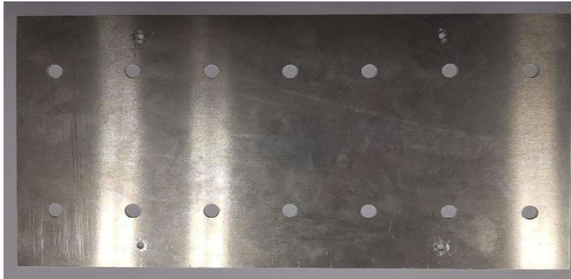
Figure 23: Mounting plate for securing the 6150AD-b to a DJI M600 (UAV).
