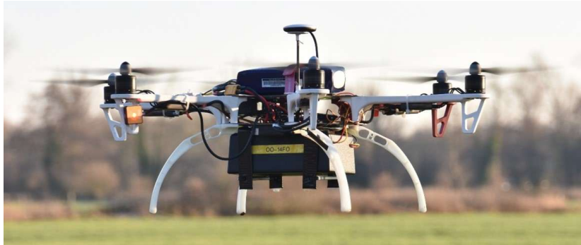
Figure 2: F550 DJI Flamewheel multicopter UAV with a payload containing a Geiger counter. Courtesy of Geert Olyslaegers.
