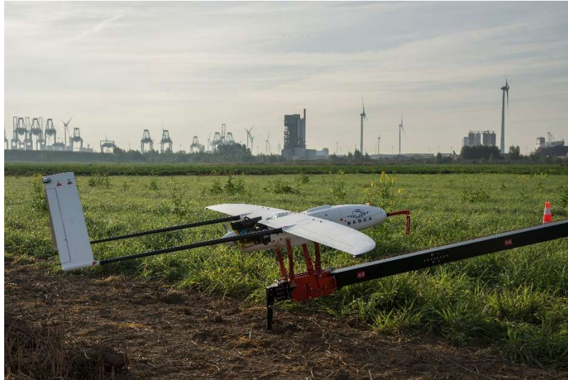
Figure 3: Penguin C fixed-wing UAV placed on a pneumatic catapult. Courtesy of SABCA.
