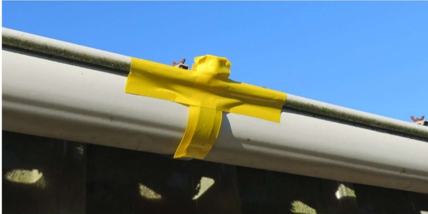
Figure 64: Cs-137 source placed on the roof of a storage building located at the SCK CEN farm. The height was approximately 2 m.
