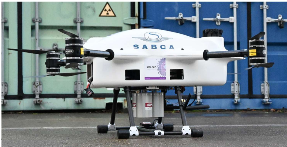
Figure 57: X8 coaxial octocopter owned by SABCA with the multicopter detector system underneath.
