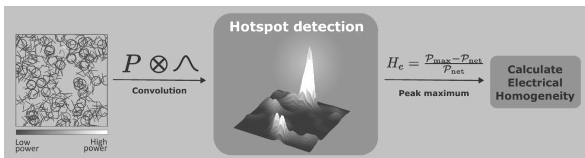
Figure 1: Strategy to calculate the electrical homogeneity. In the left image, we see a few wires that have a high power value. Using the convolution method, we are able to detect these hotspots (center image). The result of this convolution operation (and its corresponding power density) is used to calculate the electrical homogeneity measure.
