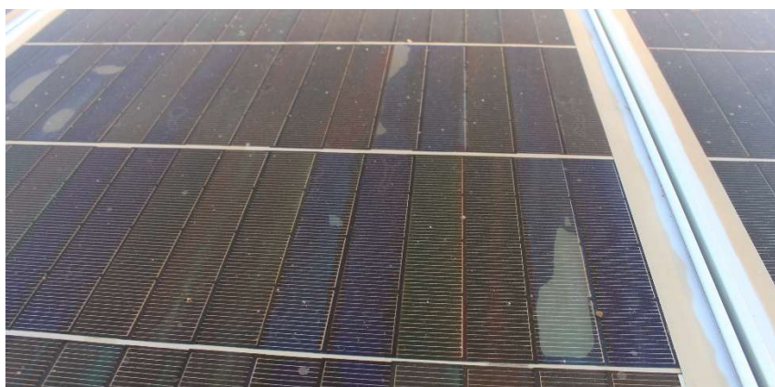
Figure 6. Delamination between the front layers in the PV stack.
