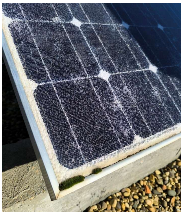
Figure 5. The glass breakage due to hail impact and the moss growing in the corner, the PV module is still producing electricity under monitored conditions.
