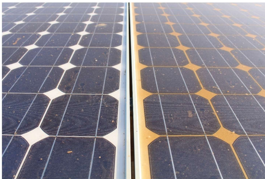
Figure 4. The presence of the yellowing of the backsheet and the soiling layer on the PV module [27].
