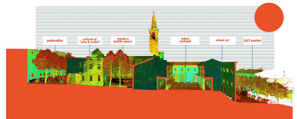
Point cloud section of the San Francesco Convent complex, Cagli, Pesaro-Ubino, Marche, Italy. Image by authors.
