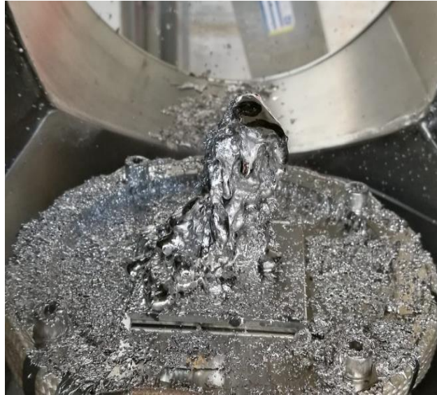
Figure 41: Pile of stacked solidified droplets with a pseudo-wet dimple at the top.
