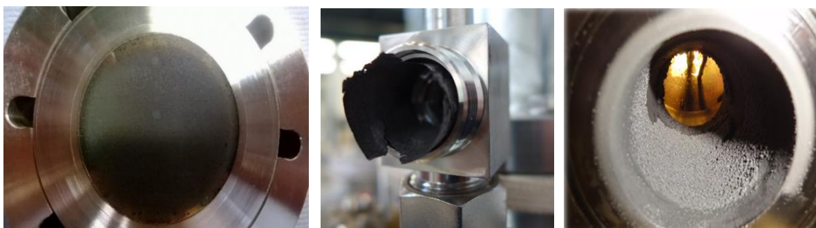
Figure 1: Presence of LBE aerosol particles in an experimental installation at the SCK CEN which uses LBE. From left to right: deposition on viewports, on filters, and in piping systems.
