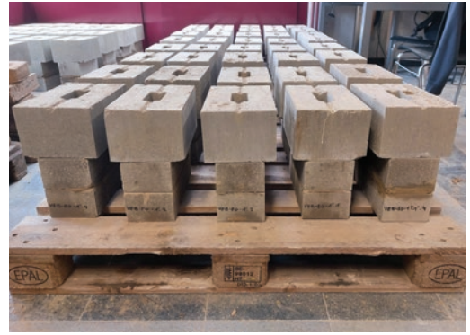
figure 2: Lab experiments on the reclaimability of earth blocks [Photo: Erik Pelicaen]
