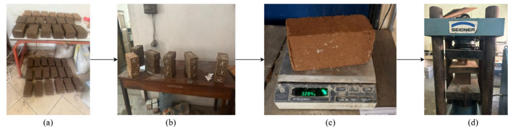
Figure 10. Testing procedure of stabilised earth blocks: (a) curing of earth blocks; (b) labelling of specimens (three per group, labelled as X, Y, and Z); (c) measurement of block weight; (d) compressive strength testing.
