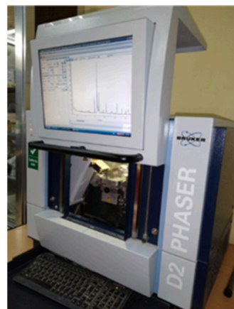
Figure 9. X-ray diffractometer (Bruker D2 PHASER) used for mineralogical analysis.
