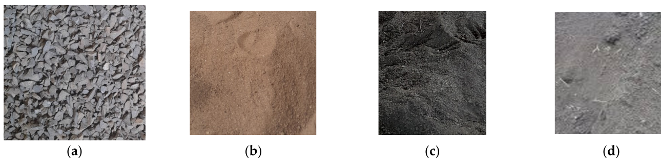
Figure 1. Raw materials used in the concrete mixes. (a) Crushed Stone (coarse aggregate); (b) River Sand (fine aggregate); (c) Steel Slag (fine aggregate and binder); (d) Sugarcane Bagasse Ash (binder).
