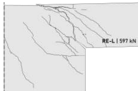
Figure 6. RE-L crack pattern at failure
