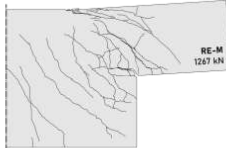
Figure 8. RE-M crack pattern at failure
