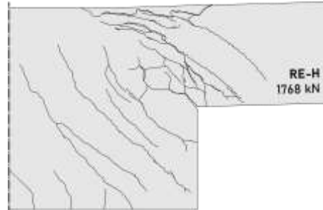
Figure 10. RE-H crack pattern at failure
