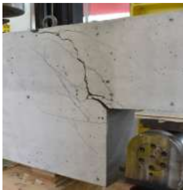
Figure 12. Failure of RE-L
