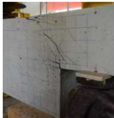
Figure 13. Failure of RE-M
