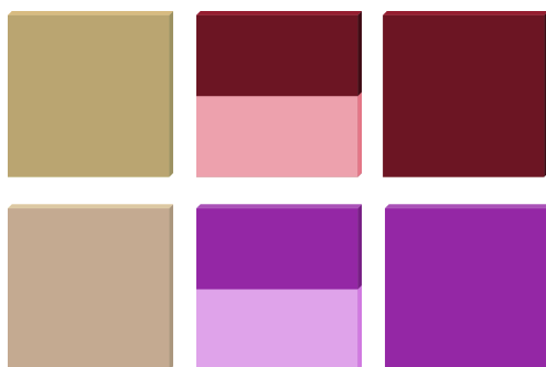
Figure 5.2: Schematic representation of the types of photo-anodes prepared for this work. From left to right: unstained control cells (C.), half-half PV photographs (HH.), and stained references (St.). The top row (in red) represents transparent SC, while the bottom row (in purple) represents opaque samples.
