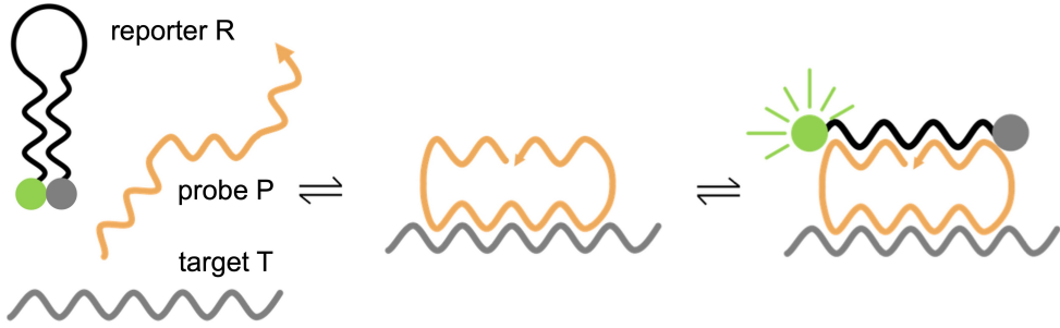
Figure 5.2: Simplified reaction diagram of the two-step process. Only after the selective binding of probe P to target T can the reporter interact with the PT complex to form the detectable, fluorescent PTR complex.
