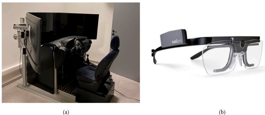
Figure 3. Experimental equipment (a) Simulator (b) Eye tracker [31].
