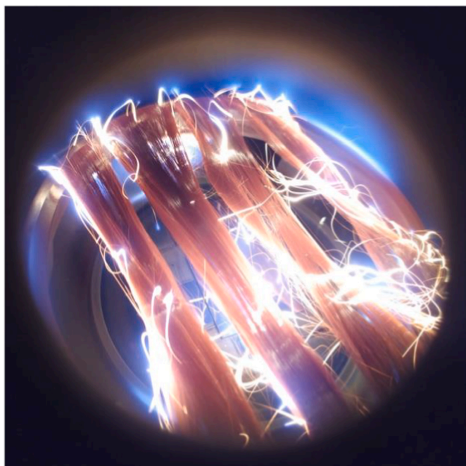
Fig. 2. CF tow inside a MW PE CVD chamber during a diamond growth process. The different colours of the CFs that compounds the tow evidence the wide range of temperature of the CFs substrates. (For interpretation of the references to colour in this figure legend, the reader is referred to the Web version of this article.)
