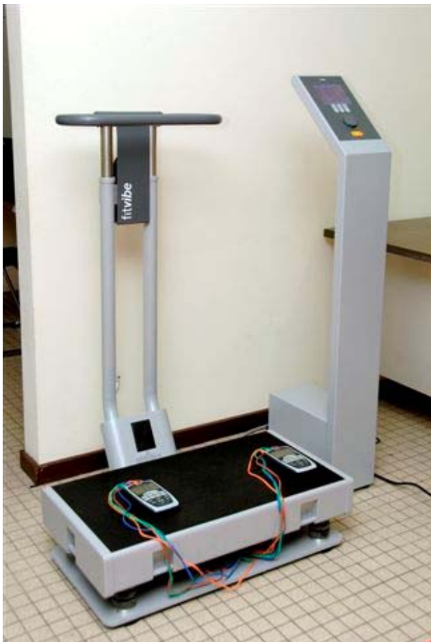
Fig.1. FitVibe ® for Whole Body Vibration (left) and operation panel (right) with electrostimulation devices lying on the vibration platform
