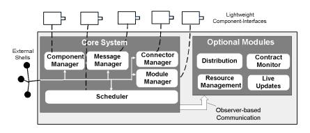
Fig. 2. High-level design of the DRACO runtime system
