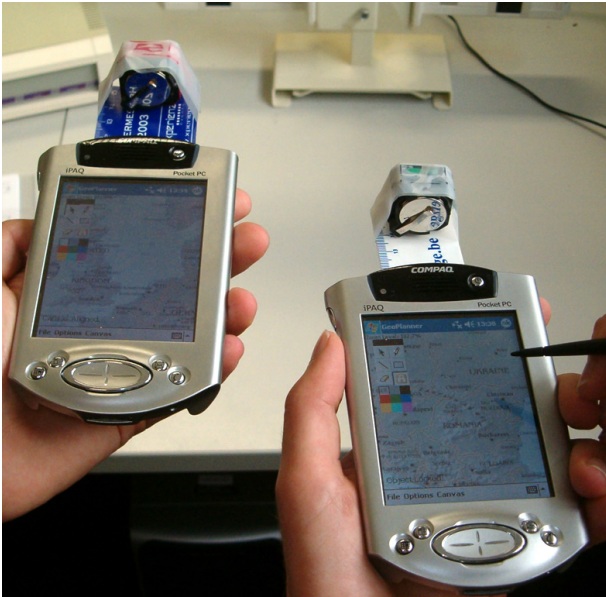
Figure 5: Two portable personal displays running the GeoPlanner application. The V-scope sensors attached on top of the PPDs are used to track them in physical space. A map of Europe was added to the shared information space. Both users can move their PPD to see other places on the map. It is also possible to zoom by moving the PPD up or down. The drawing palette on the left side of the screen offers the possibility to make annotations to the image.
