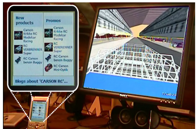
Fig. 5 The shopping buddy (implemented on a PDA) creates a mashup of nearby smart products and is coupled to the 3D simulation.
