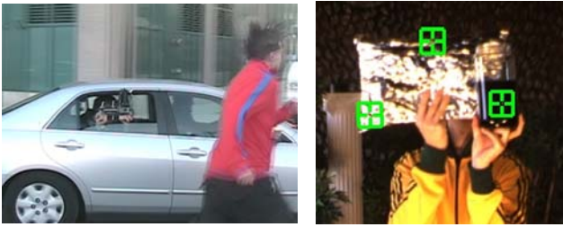
Figure 10: Robustness under different conditions. (Left) Shooting from a moving car in daylight. (Right) Highly specular scene: Three tags are attached behind aluminum foil. We track tags behind a bottle of Coca-Cola.
