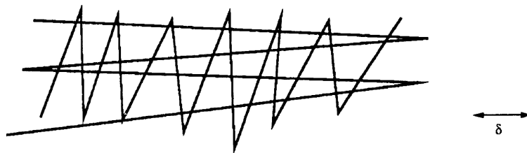
Figure 5.1: Two trajectories with Hausdorff Distance \delta , although they are far from similar, they have a very little Hausdorff Distance [AG95].
