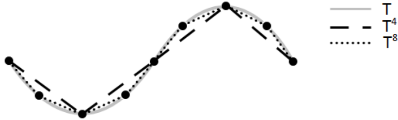
Figure 3.1: The curved line T is approximated by T^4 and T^8 . It is clear that the higher the n in T^{2^n} , the better the approximation.
