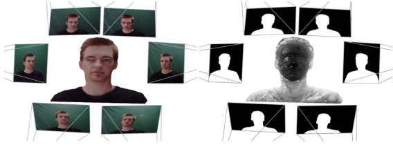
Figure 4: The view interpolation module generates a virtual image and joint depth map.
