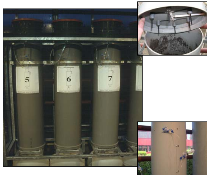
Figure 1.1 Picture of soil columns with a detail of the rainfall simulation system and pore water samplers.
