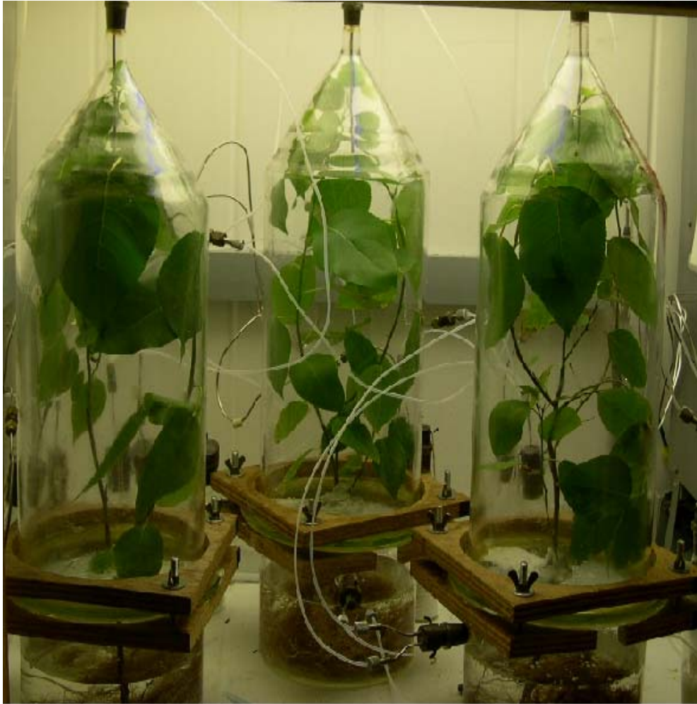
Figure 7.1: Two compartments glass cuvettes system for measurement of toluene evapotranspiration.
