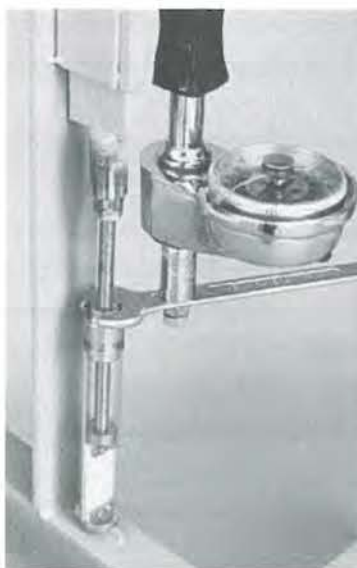
Figure 4.8: The stretching device fixed in the holder to load the specimen by use of the spanner and the torque.
