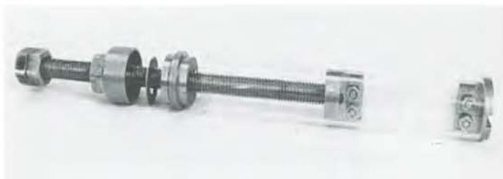
Figure 4.7: The stretching device which fits into the NMR probe head.
