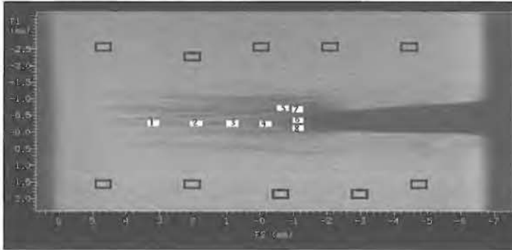
Figure 4.16: Image of ABS showing the fixed spatial locations where the spin density ( M_0 ), T_{1H} and T_{2H} relaxation times were determined. For values see Tables 4.2 and 4.3. All picture elements are 0.16 \times 0.31 mm in dimension. The reference spots (black rectangles) have a similar dimension and are located at least 1.5 mm from the damage bands.
