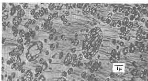
Figure 4.4: Transmission electron micrograph of ultrasection of high impact polystyrene deformed to small strain and stained with osmium tetroxide. Crazes and rubber both stain. Reproduced of R.P. Kambour 48
