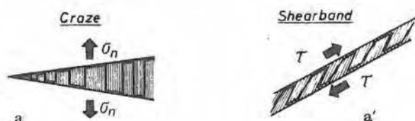
Figure 4.2: Schematic comparison of the deformation processes in crazes (a) and shear bands (a').
