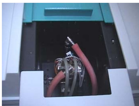
Figure II.9 B: Harrick High Temperature cell (HHT-cell) positioned in the beam of the UV-Vis spectrophotometer.
