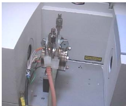
Figure II.5: Harrick High Temperature cell (HHT-cell) inserted in the beam of the FT-IR spectrometer.
