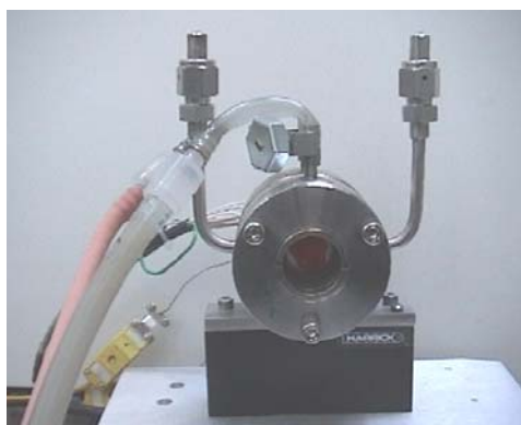
Figure II.4: Infrared Harrick High Temperature cell (HHT-cell).
