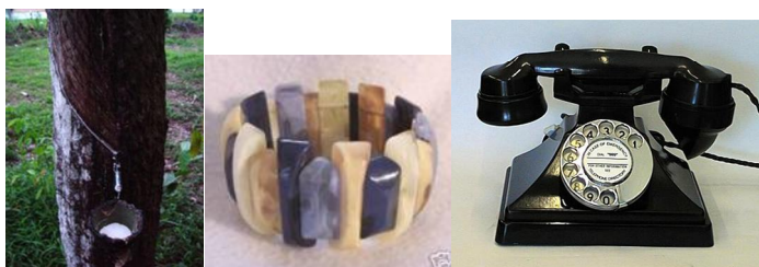
Figure 1.1: (left to right) natural rubber, semi-synthetic Galalith and a fully-synthetic Bakelite phone
