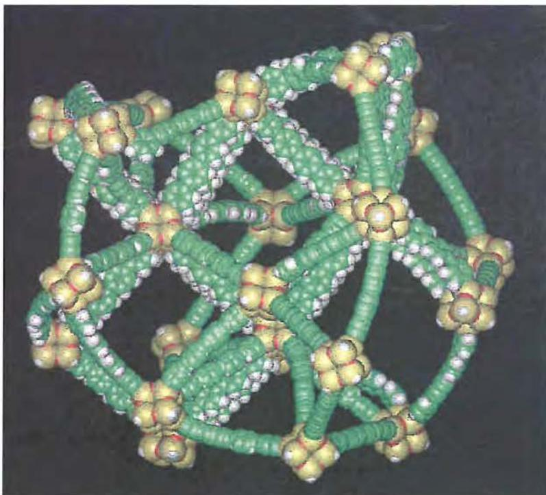
**Figure 1.9:** Configuration average at 300K of random structure as obtained after a simulation annealing run with  $T_{\text{start}} = 1500$  and  $T_{\text{end}} = 300$  K
