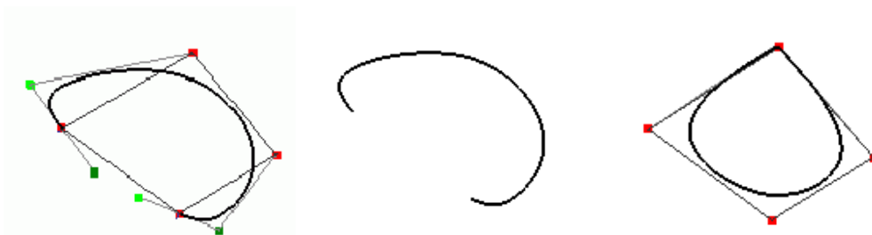
Fig. 6-7. The same technique can be applied to control normal and tension at the ends of an open curve. Left: The control vertices and ghost points. Center: The resulting open curve. Right: Connecting the ends of an open curve allows the creation of a closed curve with a sharp corner.
