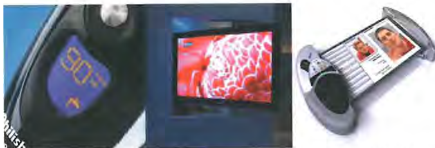
Figure 3. (a) the James Bond 007 shaver with a OLED display (Philips®) 38 (b) 31-inch OLED TV (Samsung®) 39 and (c) Mobil phone with a integrated rollable OLED display (Polymer Vision®). 40
