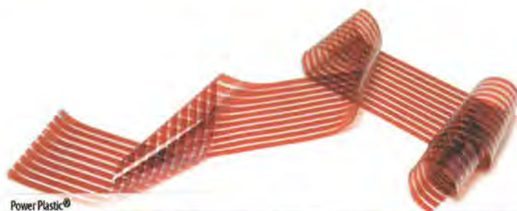
Figure 2. a) polymer inks (BASF electronics®) 15 b) roll to roll printing on flexible substrates (PolyIC®) 16 c) a flexible and light weight organic solar cell. (Konarka's PowerPlastic®). 17
