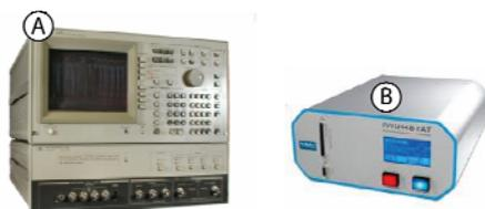
Figure 5-1: A) 'HP4194A impedance/gain-phase analyzer', from Hewlett-Packard, USA
