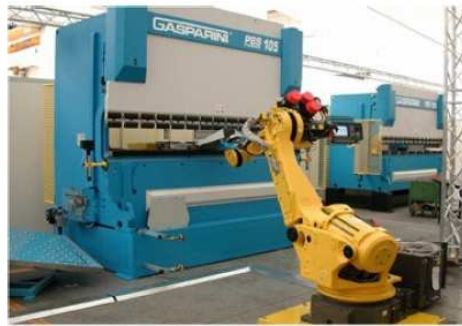
Figure 4.1: A robot assisted sheet metal bending system. Image courtesy of FANUC robotics.
