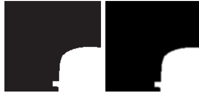
Figure 2.9: Simple alpha map construction, by convolution of a binary layer mask with a Gaussian kernel.
