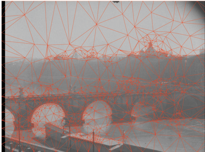
Figure 2.4: Motion adaptive warping mesh, superimposed on a reference frame from a panning sequence. By weighing the candidate vertices with the image gradient, nodal points are placed on strong image features.
