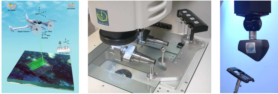
Figure 2.12: Some typical examples of scanning methods. From left to right: Airborne LIDAR sensing, touch probe acquisition and laser scanning. Photographs courtesy of NASA, Institut de Production et Robotique and Metris respectively.
