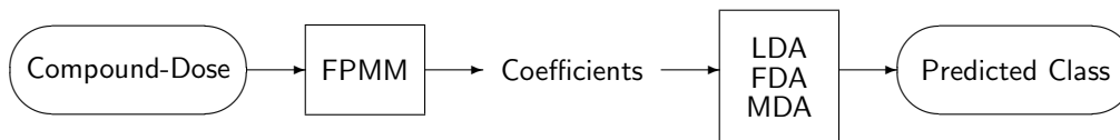
Figure 6.1: Diagram representing the doubly hierarchical discriminant analysis, when a fractional polynomial mixed model (FPMM) is used in Stage I and linear (LDA), flexible (FDA) or mixture discriminant analysis (MDA) are used in Stage II.
